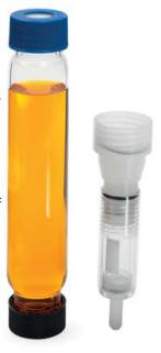
Works in combination with the Puck to enable direct concentration into a 2ml GC vial
